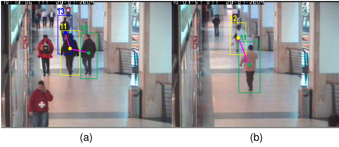
Fig. 4. Two examples (a) and (b) generating incorrect elementary groups if the distances are not normalized.
